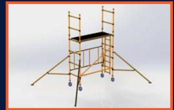
**7:** Fit the platform on the 4th rung ensuring the hatch is facing the ladder frame.
