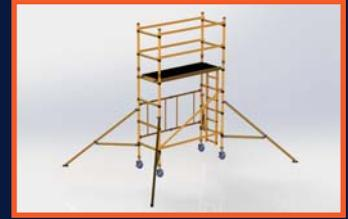
**8:** Using the 3t method place horizontal braces on the 5th and 6th rungs.
